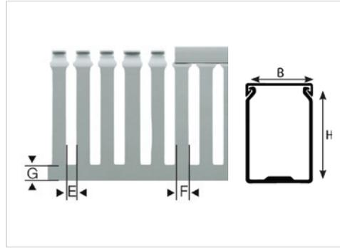
Iboco TD range features a 12.5 module according to DIN 43659 and CEI 23-22 standards which is particularly suitable for use with other DIN 12.5 equipment for perfect size interfacing. Optimised duct size/wire retention ratio and perfectly rounded finger edges for safe operations even in installations with difficult access. Repeated opening and closing of the fingers during wiring operations is possible due to their size and resilience.
