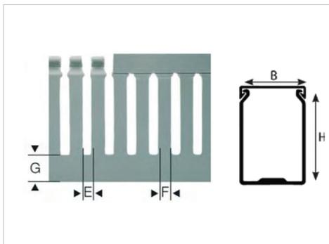
Iboco T1-E range is commonly employed in electric control panels. It has restricted slot opening and its strong and robust due to its thick base and side construction. Perfect solidity is also guaranteed in cantilevered applications. Made of material with more than 3000NPa modules of elasticity, it allows for repeated opening and closing of the duct fingers during wiring operations even at low temperature, without breaking.
