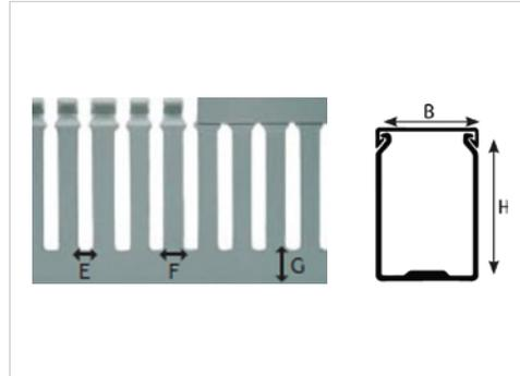
Iboco T1-EF range is ideal for small sized wires commonly employed in electric control panels. It has restricted slot opening and its strong and robust due to its thick base and side construction. Perfect solidity is also guaranteed in cantilevered applications. Made of material with more than 3000NPa modules of elasticity, it allows for repeated opening and closing of the duct fingers during wiring operations even at low temperature, without breaking.
